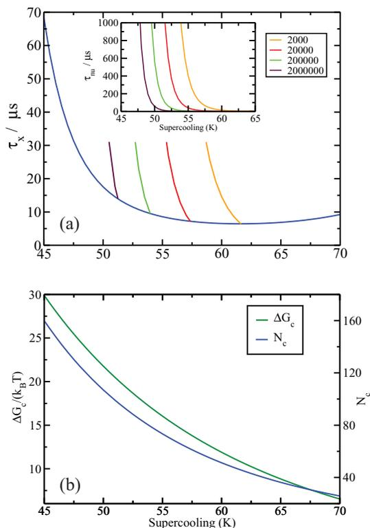
FIG. 9. (a)  $\tau_x$  for  $\phi = 0.7$  for the TIP4P/2005 model as a function of the supercooling.  $\tau_x$  is the time necessary to crystallize 70% of the system. Inset: plot of the nucleation time,  $\tau_{nu}$ , versus the supercooling. (b) Free energy barrier for nucleation and size of the critical cluster for TIP4P/2005 as a function of the supercooling.
