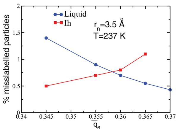
FIG. 1. Percentage of mislabelled particles according to  $\bar{q}_6$ , evaluated for bulk ice Ih and bulk liquid water at 237 K and 1 bar (for TIP4P/2005), using the first minimum of the  $g(r)$  (i.e.  $r = 3.5$  Å) as a cutoff for the calculation of  $\bar{q}_6$ . For ice Ih, mislabelled particles are those with a value of the order parameter smaller than  $\bar{q}_6$ . For liquid water, mislabelled particles are those with a value of the order parameter larger than  $\bar{q}_6$ .
